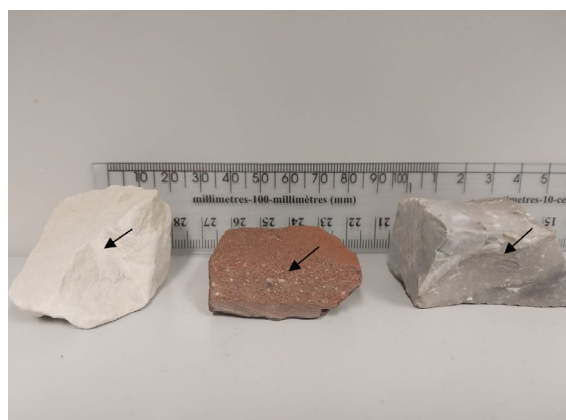
Figure 1. Tested rock samples. Chalk (left), haematitic oolite (centre) and chert (right). The arrows indicate where test portions were extracted for destructive analyses.
