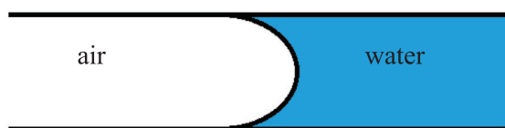
FIGURE 1 A single interface between water and air in a capillary tube.
